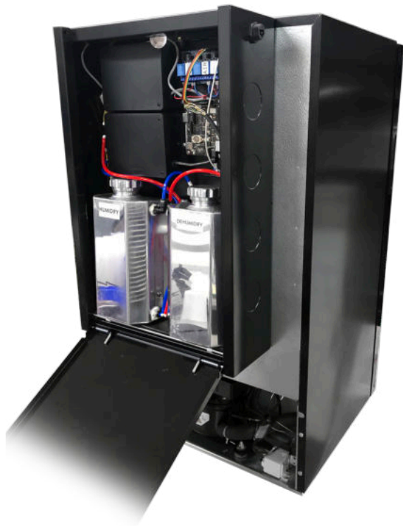
Locked Control Cabinet on Rear of Unit (Open) with Desiccant and Humidity Canisters
